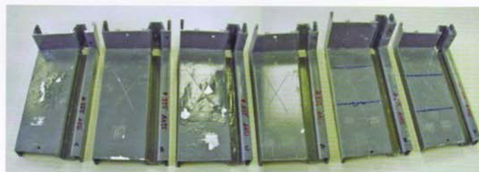
Samples after 1000 hour Acetic Acid Salt Spray Test
